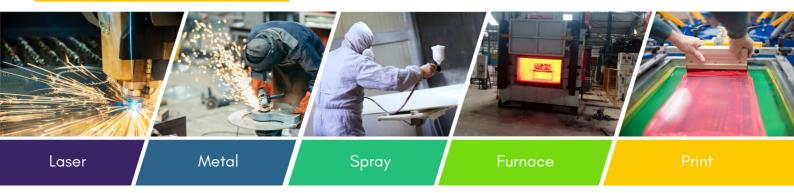
Enamel panels are cut out of low-carbon steel using our fibre lasers; they're then formed into the panels before being degreased. The milled enamel coating is then sprayed on and fused to the steel before and prints are added.
