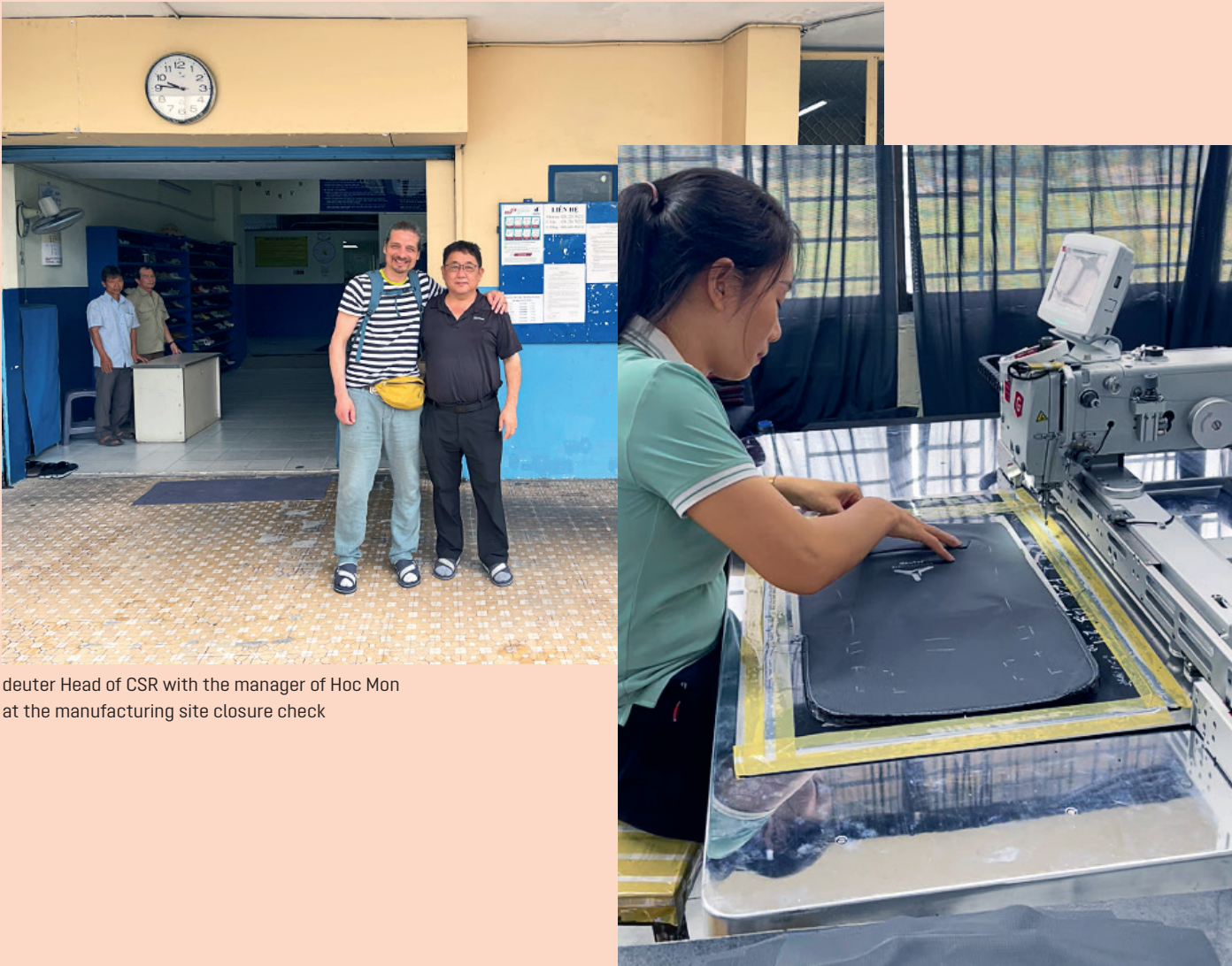
Computerized sewing machines for automated back panel stitching
